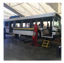
The chassis is stripped down to the frame, once the bus has been qualified as structurally sound.
