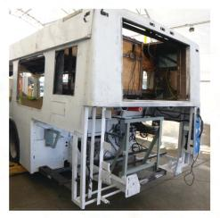
The diesel engine and related components, including the transmission, are removed.
