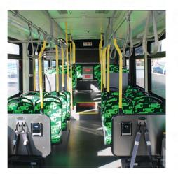
New composite flooring, lightweight seating, and LED interior/exterior lighting is installed.
