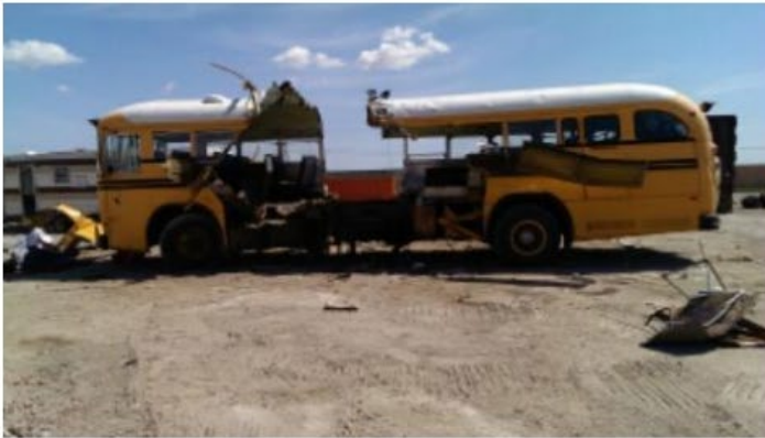
Example of acceptable destruction of vehicle chassis
