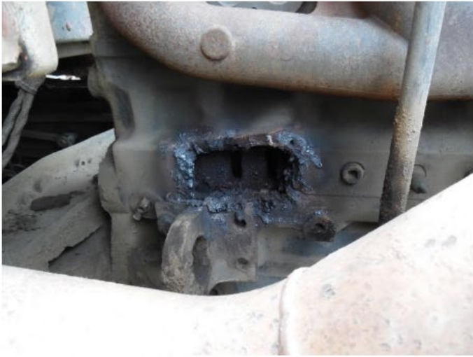
Engine: 5" hole in engine block
