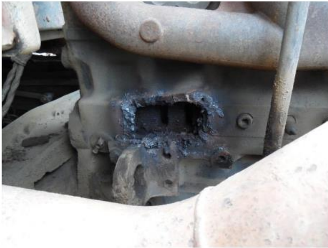
Engine: 5" hole in engine block
