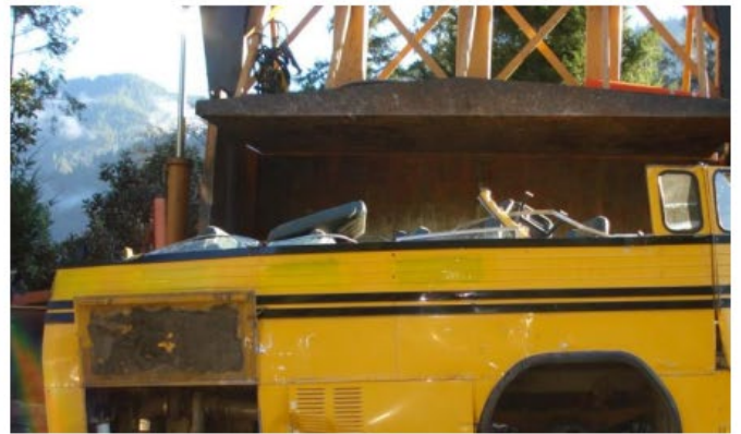
Example of acceptable destruction of vehicle chassis
