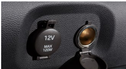
12 V Dual Power Outlets
