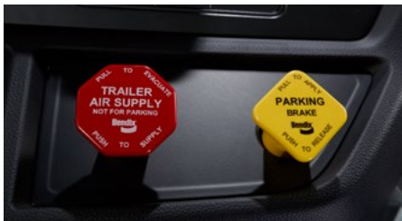
Trailer Air Supply and Parking Brake Switches
