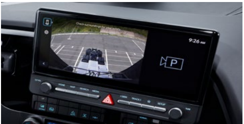
Deck View Monitor Equipped with an extra-wide-angle lens, the screen provides a real-time rear view video feed.
