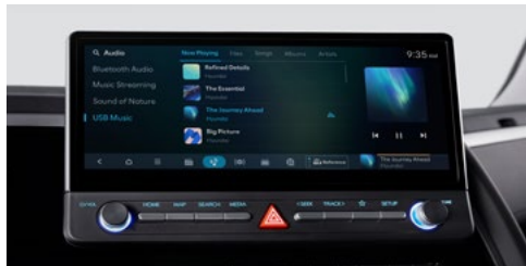
Intuitive 12.3-inch Touchscreen Directly below the head unit, a row of physical buttons flanked by rotary control dials serves as one-touch shortcuts to access the most commonly utilized functions.
