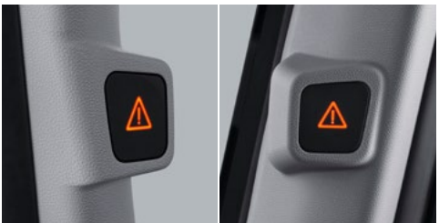
BCW* & BCW-Near Indicators The BCW & BCW-Near indicators are positioned on both front pillars for optimal visibility. * Blind-spot Collision Warning
