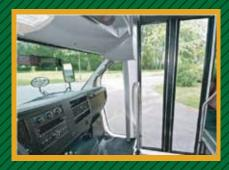
Maximum visibility of loading zone is provided by fully-glassed entrance door and unobstructed "More-View" window. Standard 32" electric double-opening door.
