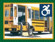
Special needs Micro Bird with double-leaf wheelchair doors offer protection on both sides of the lift, thus adding to passenger safety, while offering superior weather seal and door strength.
