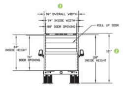
The box dimensions and configurations on this page represent a standard dry freight box. The liftgate as pictured is an option and not part of the standard configuration.
