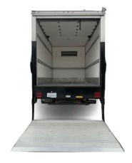
EV Star Cargo Plus has 836 cubic feet of cargo capacity.
