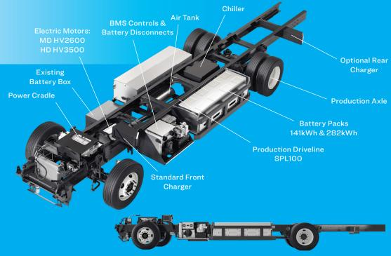
The **power electronics cradle** includes the vehicle's on-board charger, battery disconnect controls, vehicle software, cab heater unit and air compressor. The cradle is located in a single, easily accessible service point, where a traditional diesel engine would be located.
